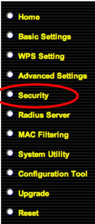
The access point provides a variety of wireless security options (wireless data encryption). When data is encrypted, information transmitted wirelessly cannot be read by anyone who does not know the encryption key.
