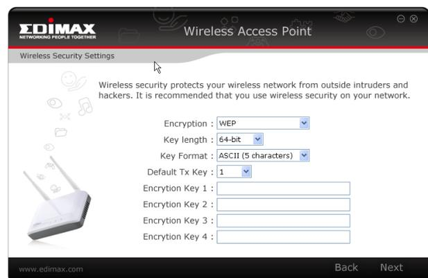
The screenshot shows the 'Wireless Security Settings' page with 'Encryption' set to 'WEP'. Below this, there are dropdown menus for 'Key length' (set to '64-bit') and 'Key Format' (set to 'ASCII (5 characters)'). There is also a dropdown for 'Default Tx Key' set to '1'. Below these are four empty text input fields for 'Encryption Key 1', 'Encryption Key 2', 'Encryption Key 3', and 'Encryption Key 4'. A router image is on the left, and 'Back' and 'Next' buttons are at the bottom right.
