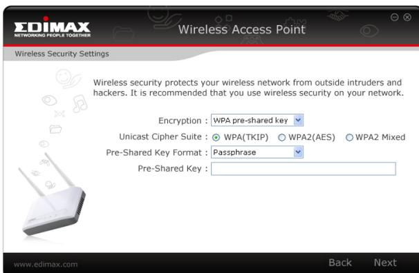
The screenshot shows the 'Wireless Security Settings' page with 'Encryption' set to 'WPA pre-shared key'. Below this, there are radio buttons for 'Unicast Cipher Suite' with 'WPA(TKIP)' selected, and 'WPA2(AES)' and 'WPA2 Mixed' unselected. There is also a dropdown for 'Pre-Shared Key Format' set to 'Passphrase' and an empty text input field for the 'Pre-Shared Key'. A router image is on the left, and 'Back' and 'Next' buttons are at the bottom right.
