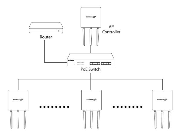
**4.** Connect a computer to the designated AP Controller using an Ethernet cable.
