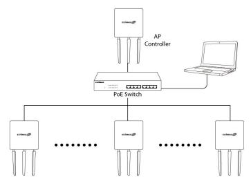
2. Open a web browser and enter the AP Controller's IP address in the address field. The default IP address is **192.168.2.2**
