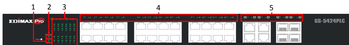
Figure 4 – GS-5424PLC Front View LED Indicators
