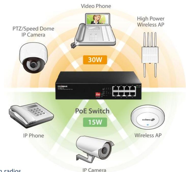
\*IP Phone: 3- 7W, IP Camera: 7- 10W PZT Camera: 15 -25+ W
