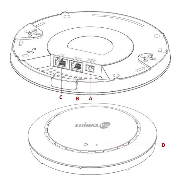
A 12V DC IN 12V DC port to connect the power adapter
