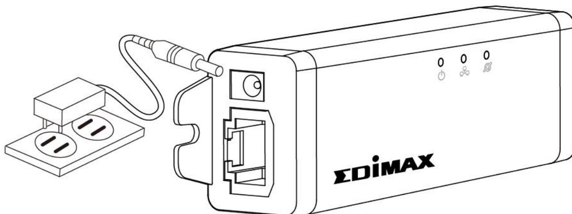
**11.** You can use an Ethernet cable instead of Wi-Fi to connect the indoor main unit to your router/access point for more stable performance if you prefer.
