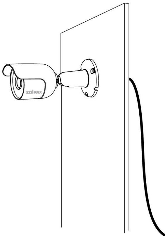
5. Use a sealant to seal the gaps around the cable and screw the outdoor image unit into place.
