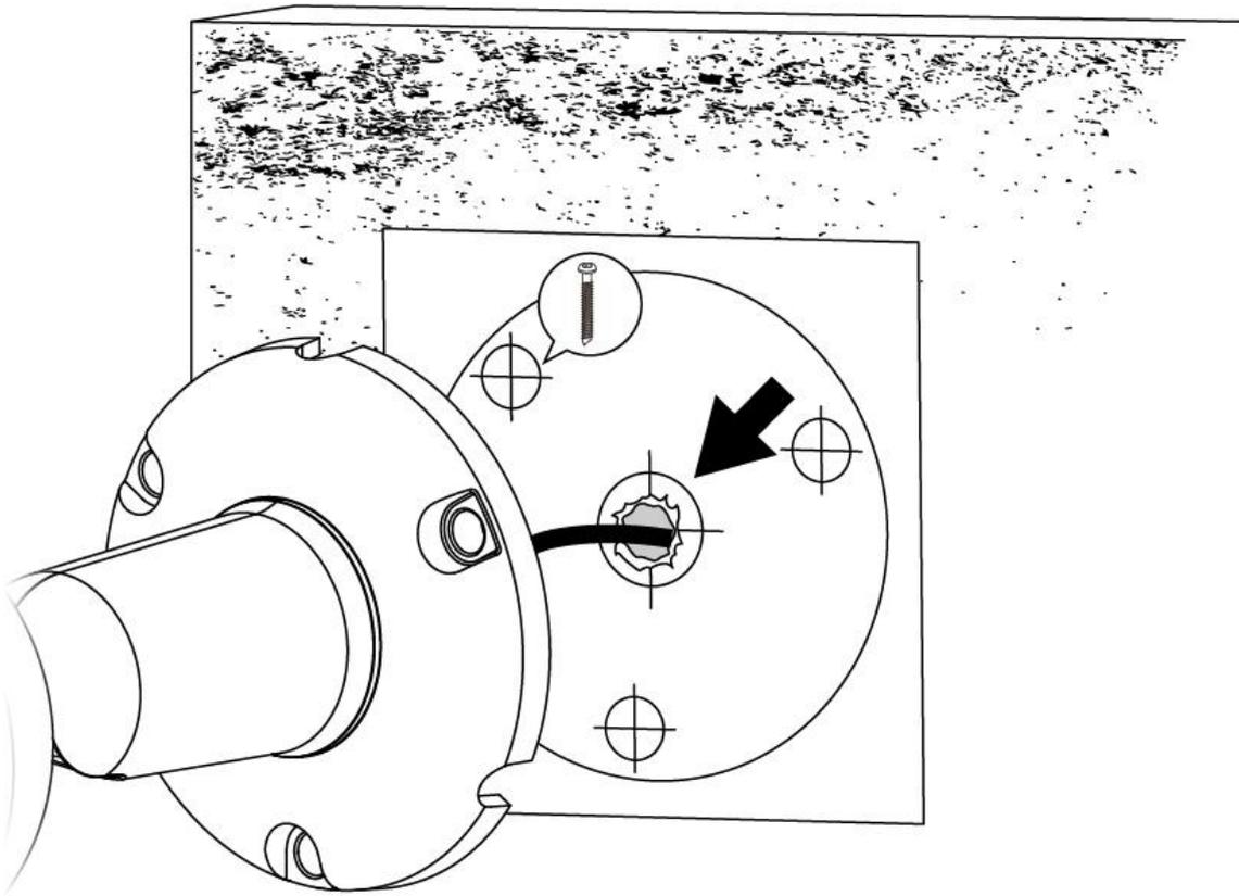
4. Run the cable attached to the outdoor image unit through the hole from the outside to the interior.
