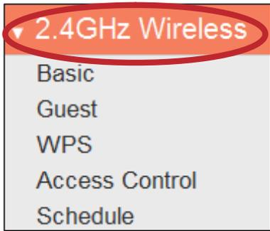
The “2.4GHz Wireless” & “5GHz Wireless” menu allows you to configure SSID and security settings for your Wi-Fi network along with a guest Wi-Fi network. WPS, access control and scheduling functions can also be managed from here.
