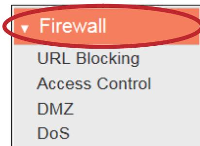
The “Firewall” menu provides access to URL blocking, access control, DMZ and DoS functions to improve the security of your wireless network.
