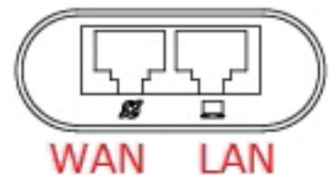
In **other** modes, both ports function as LAN ports for wired network devices (e.g. computers, games consoles etc.), and in **access point** mode also for connecting to your router.
