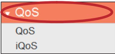
Quality of Service (QoS) is a feature to manage Internet bandwidth efficiently. Some applications require more bandwidth than others to function properly, and QoS allows you to ensure that sufficient bandwidth is available. Minimum or maximum bandwidth can be guaranteed for a specified application.
