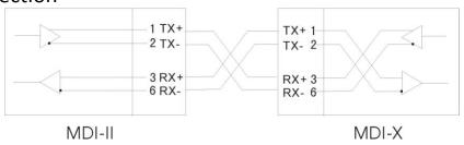
Cross over cable for switch (MDI-X port) to switch/hub or other network devices (MDI-X port) connection.
