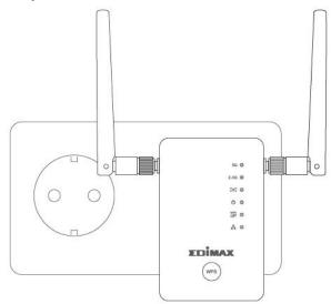
**3.** The **green** power LED will **flash** while the extender is starting up. The device is ready when the **green** power LED displays **on**.
