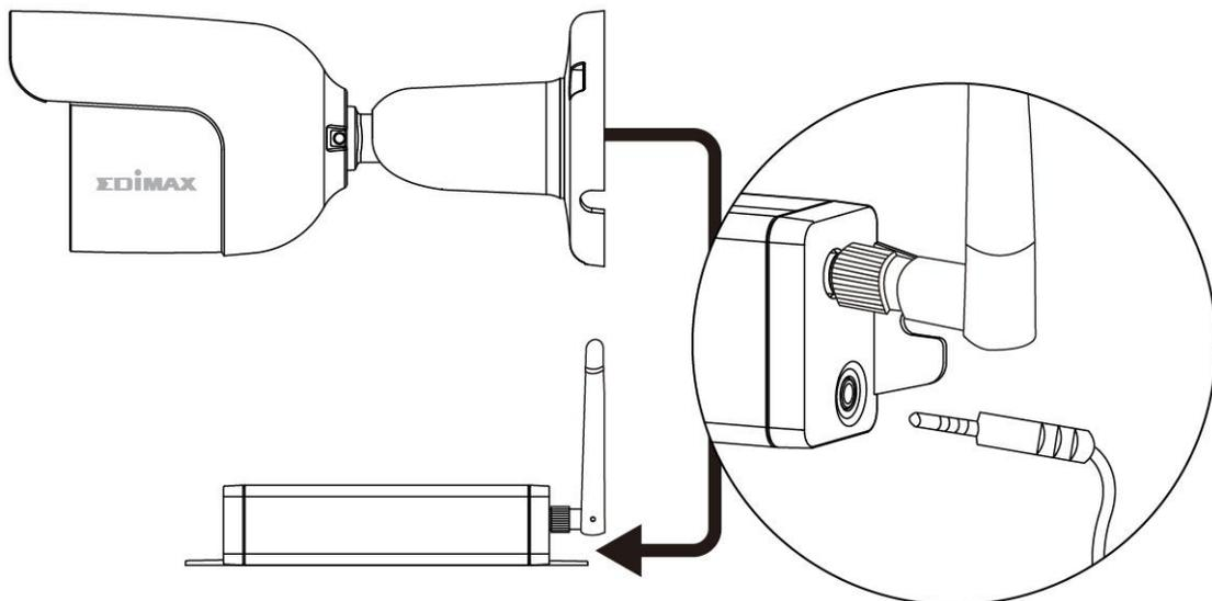
**3.** Connect the power adapter to the indoor main unit and to a power supply.
