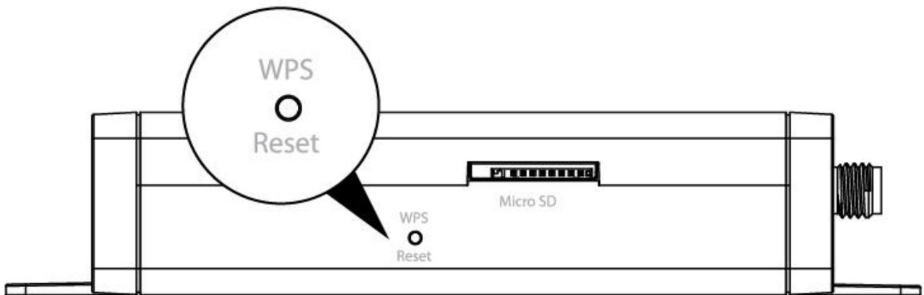
2. Release the button when the **green** power LED is **flashing quickly**.
